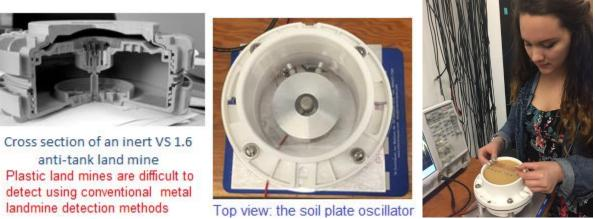
Figure 1. Left to right: VS 1.6 land mine, top view of soil plate oscillator, and co-author EVS.
