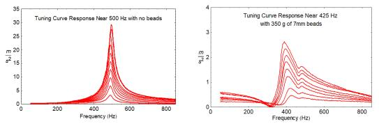
Figure 3. Aluminum SPO accelerometer response on the underside of the clamped elastic plate near the fundamental resonance of (a) the soil plate oscillator without bead loading and (b) with 7mm beads
