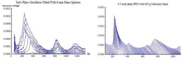
Figure 5. Comparing the tuning curve response on the underside of the clamped elastic plate (a) with 350 grams of 6 mm diam beads (b) with 634 grams of dry sifted masonry sand.
