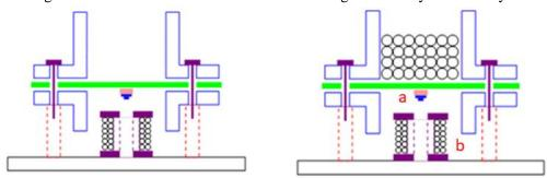
Figure 2. Left to right: Soil plate oscillator – no bead loading. Soil plate oscillator with bead loading.
