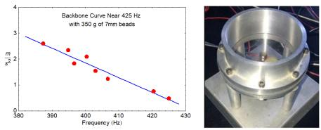
Figure 4. (a) Aluminum SPO backbone curve response on the underside of the clamped elastic plate with 7 mm diam bead loading is obtained by plotting the peak acceleration and corresponding resonant frequency from the tuning curves in Fig. 3. (b) Image of soil plate oscillator using aluminum flanges that are ½ inch thick with a circular column of 4.5 inch inside diameter and ¼ inch wall thickness
